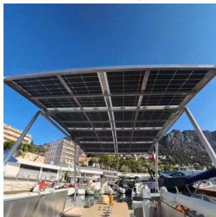
Solar canopy 1600 Wp
